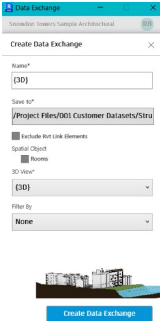
Figure 11 – Inputs to Data Exchange add-in in Revit
