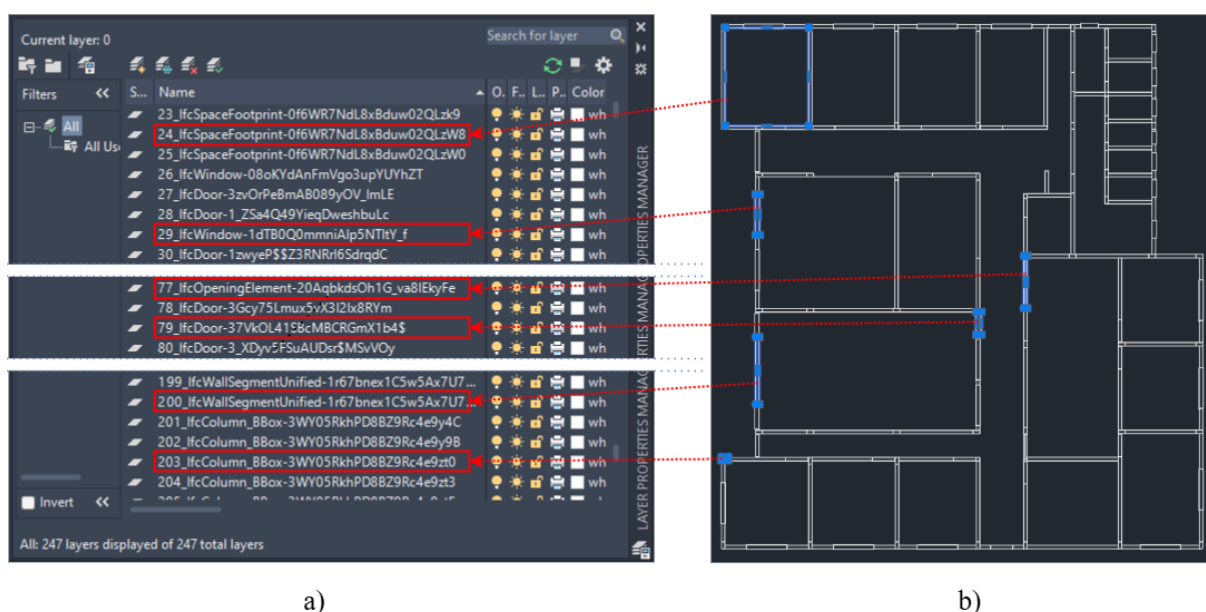
Figure 18 Visualizing CSV Coordinates in CAD Tool (b) with Corresponding Layers (a)
