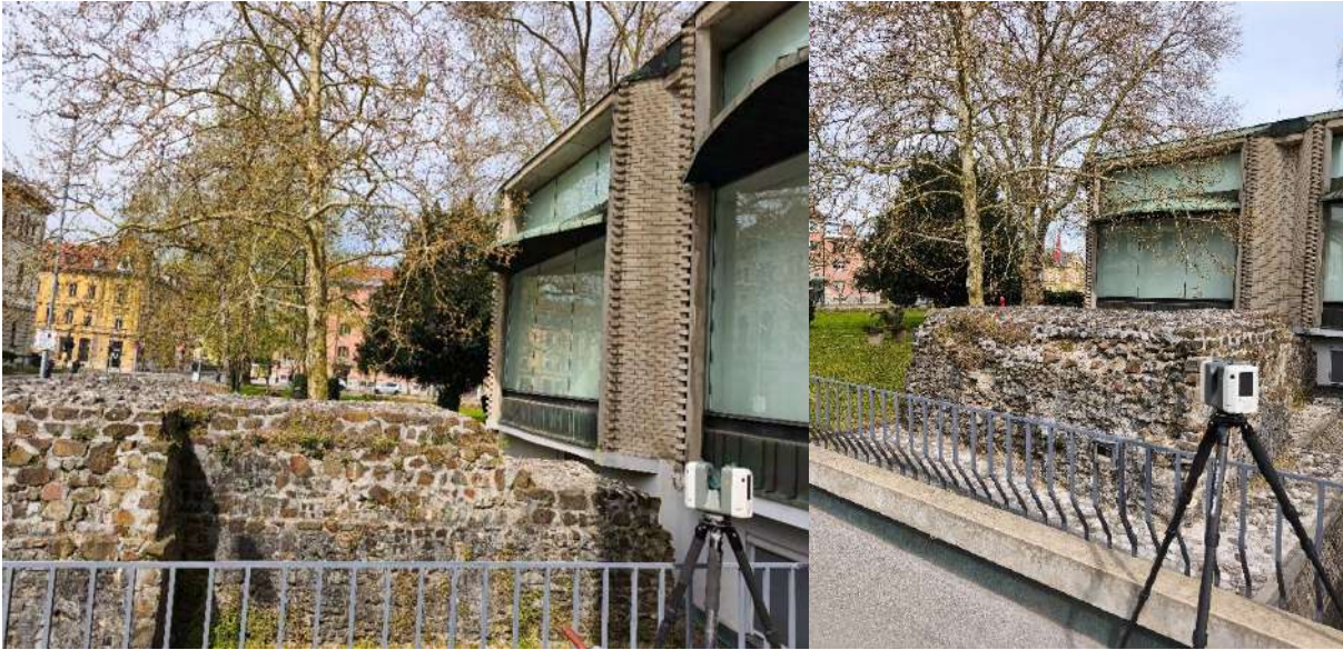
Figure 71 Two LiDAR scan positions in the EW1 section
