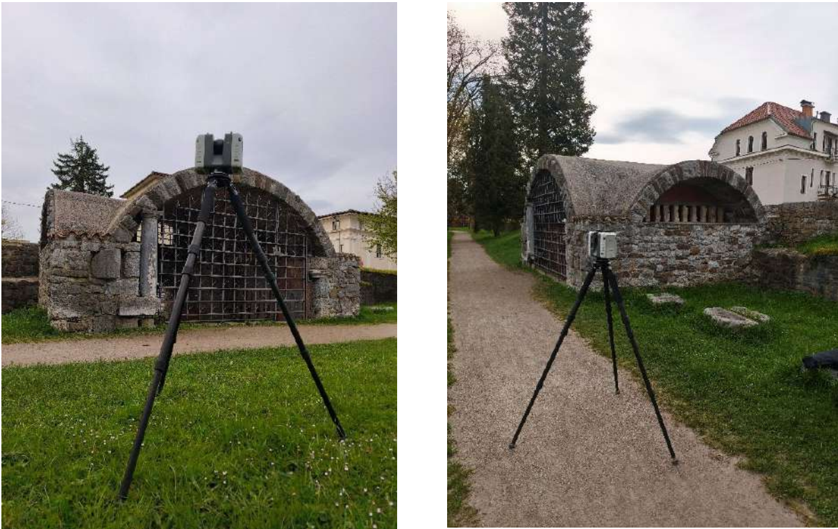
Figure 77 Re-acquiring data of the outside of the Lapidarium to enable the merging with the existing dataset.
