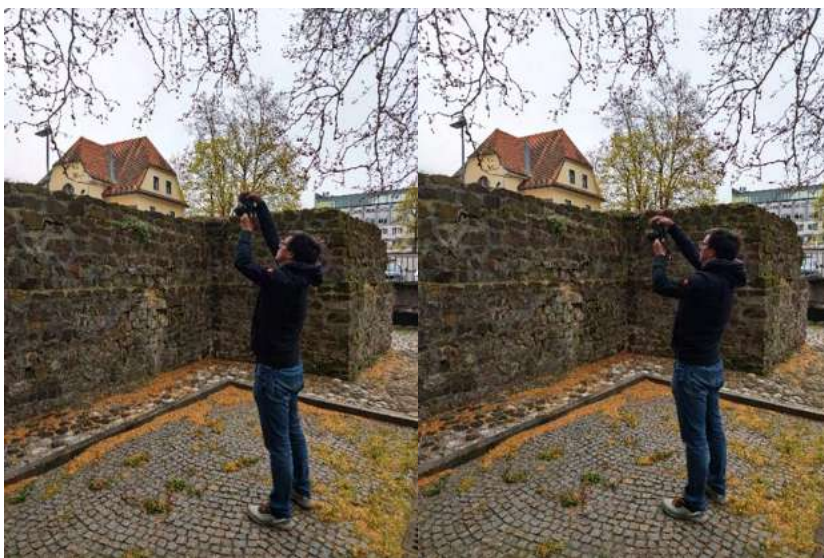
Figure 82 Example of capture from EW1 with angle variance from the same position
