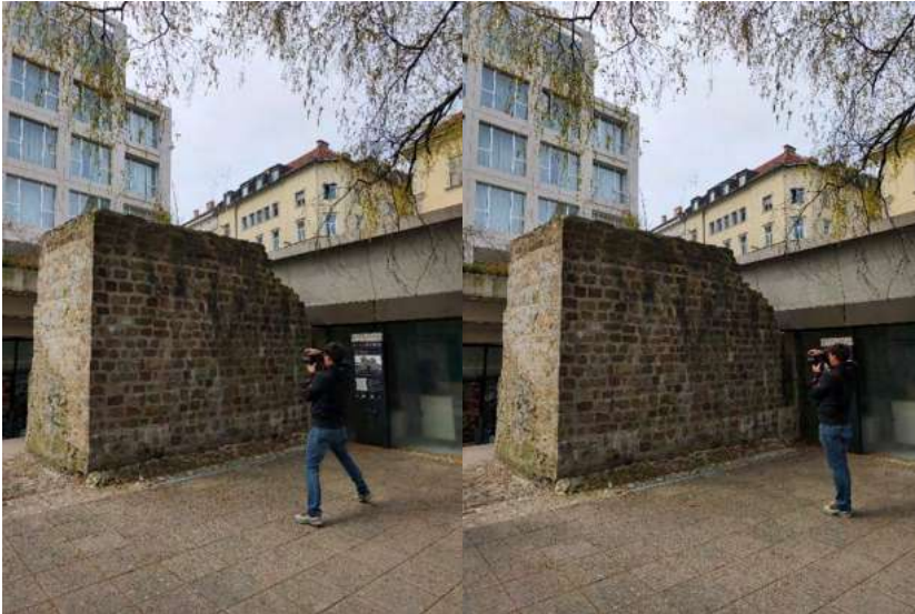
Figure 84 Example of two viewpoints capture from the EW3 with 80% overlap
