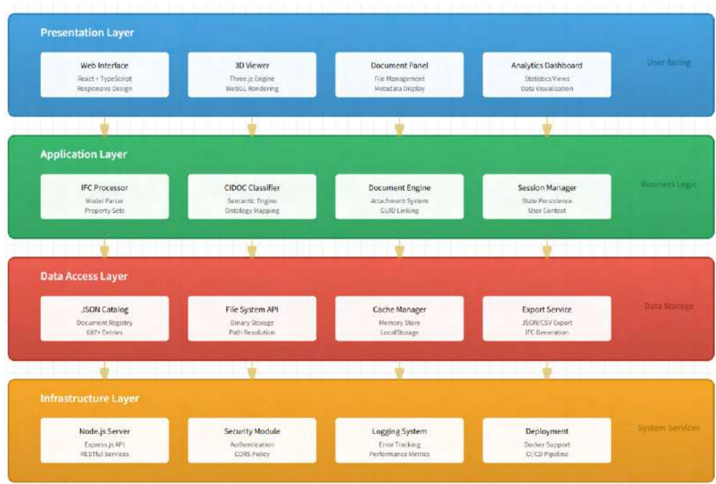
Figure 63 Four-tier architectural model showing component distribution across presentation, application, data access, and infrastructure layers (obtained from Claude)
