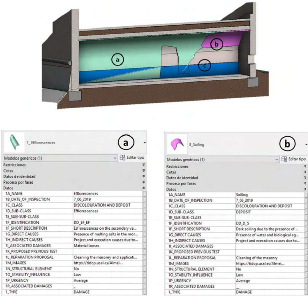
Figure 50. Damage type specimens integrated into the BIM model manually through the 3D point cloud: a) moisture in the secondary vault; b) efflorescence in the secondary vault [62]
