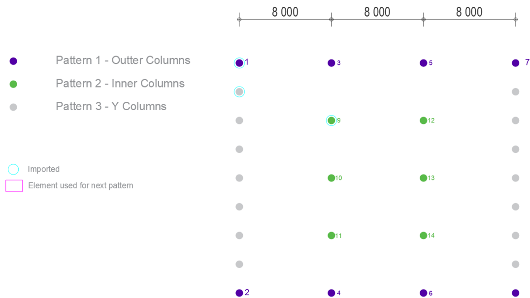
Figure 49 – Column patterns for greenhouse with one width
