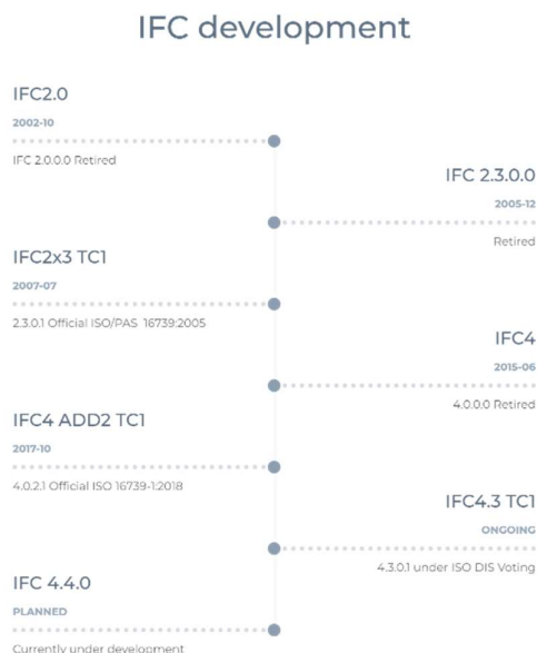
Figure 2.3 Most notable IFC schema versions through time (adapted from (buildingSMART, 2023a))
