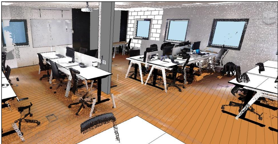
Figure 43 – Inside View of Aligned Revit Model with Point Cloud
