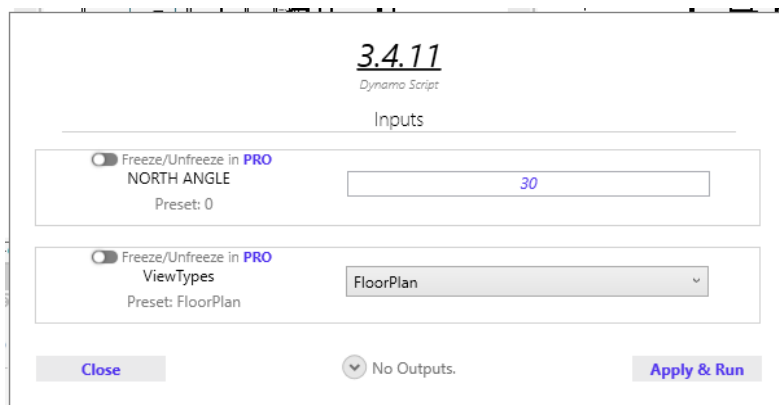
Figure 81 – Nonica pop-up to insert the inputs of the script
