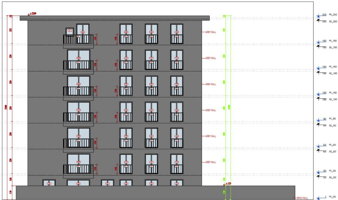
Figure 50 – Elevation view after running the script checking for overlapping between dimensions annotations and spot elevations
