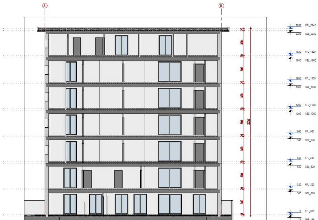
Figure 32 – Section view after running the plug-in to place annotations dimension in levels using By View mode
