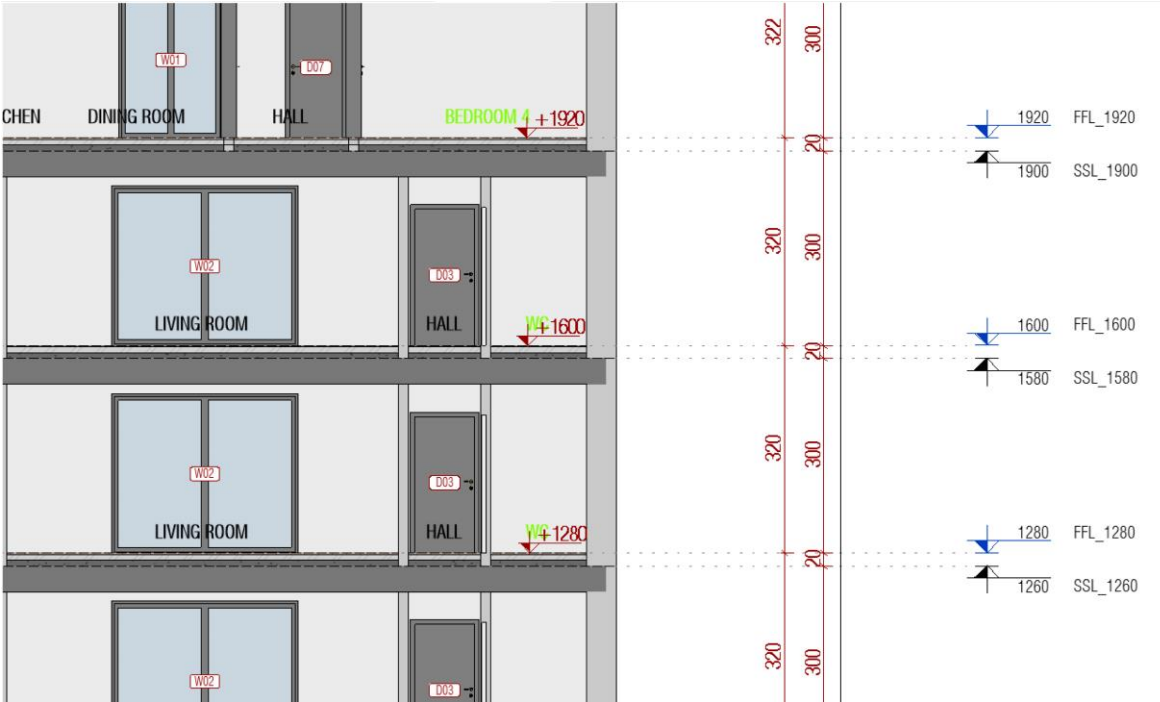
Figure 52- Section view after running the script checking for overlapping between Room tags and spot elevations
