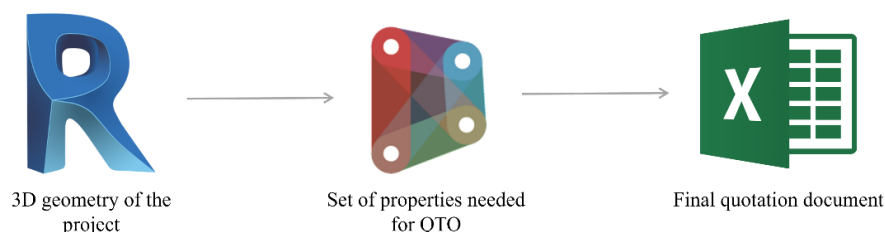
Figure 17 – Revit, Dynamo and Excel workflow. Adapted from: (Zaman & Nast, 2022)
