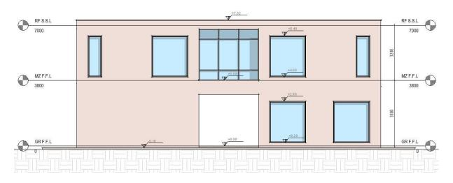
Figure 26: Back Elevation
