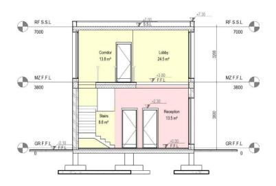
Figure 23: Cross Section 3
