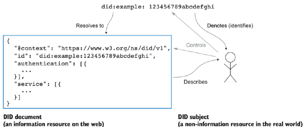
Figure 26: Relationships between DID, DID subject and DID document – Source: (Reed, Allen and Vogelsteller, no date)
