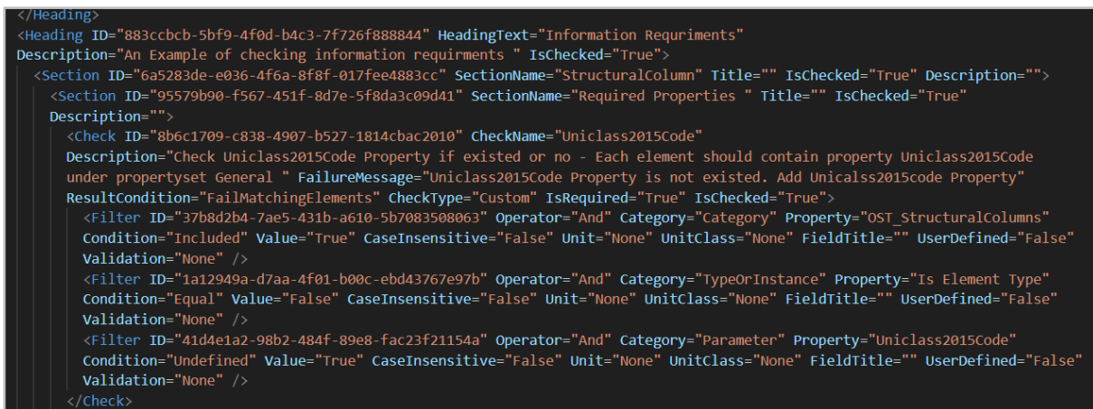
Figure 27: Autodesk Interoperability Tools – Editing checks in XML
