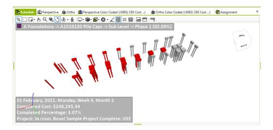
Figure 40: Elements highlighted in red to be completed as per the Look-Ahead Plan
