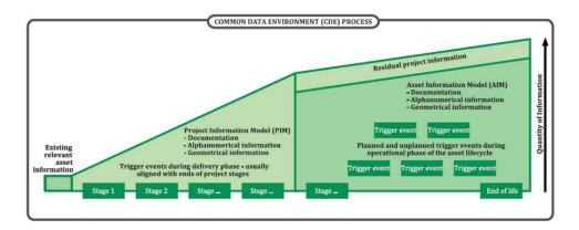
Figure 15: Data gathered during a project lifecycle according to ISO 19650-1
