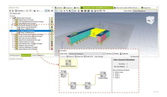
Figure 30: Selection set based on the phases of construction
