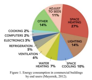
Furthermore, the end use of energy consumption in commercial buildings is a major concern, with space heating (27%), lighting (14%), space cooling (10%) and water heating (7%) being the main drivers as it is seen in Fig. 1 (Mayernik, 2012). As the major factors are all related to the actual use of buildings, the gap between the operation of a building and the actual needs of its occupants represents a potentially large opportunity for
