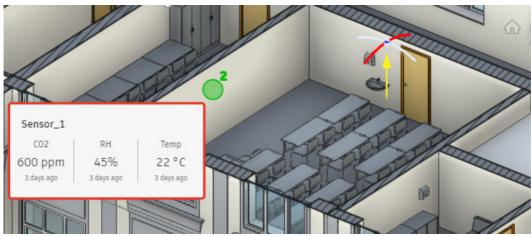
Figure 42. Data from a particular Stream
