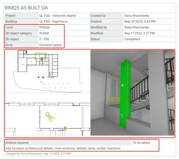
Figure 27. AS-BUILT QA checklist in Dalux Field
