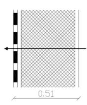
According to Zupan (2015), as for the layers of the external walls – it is slightly different from floor to floor. For the external walls of the basement there are 2 types of such layers, 510 mm and 620 mm thick:
