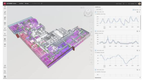
Figure 9. Heat maps of real time t °, RH, CO<sub>2</sub> levels. (Autodesk Tandem, 2021)
