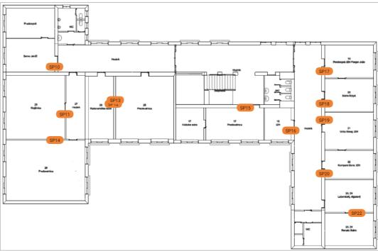
Figure 36. Placement of IAQ Sensors in the First Floor
