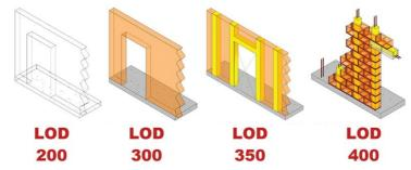
Figure 32. A masonry wall element LOD progression. (BIMForum, 2020)
