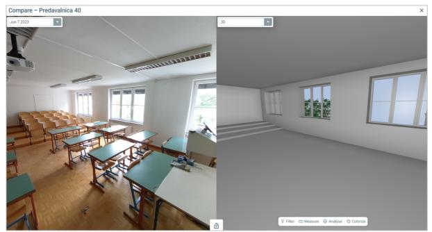
Figure 30. Comparison between 360° photos and model for the classroom 40
