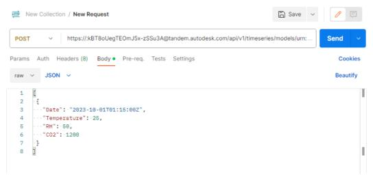
Figure 44. Data generation and transmission to Streams from Postman App
