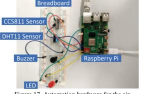
Figure 17. Automation hardware for the air quality use case (Govindasamy et al., 2021)
