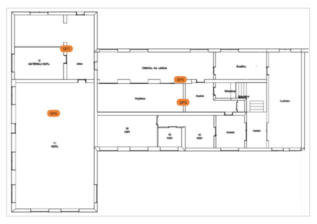
Figure 34. Placement of IAQ Sensors in the Basement
