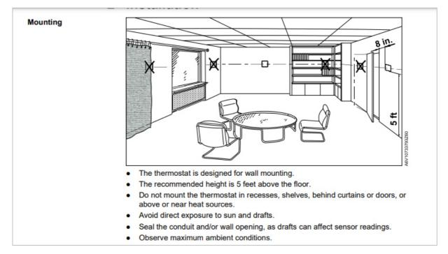
Figure 40. Example of mounting requirements for Smart Thermostat (Siemens, 2021).
