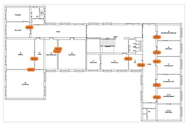
Figure 38. Placement of Occupancy/Light Sensors in the First Floor
