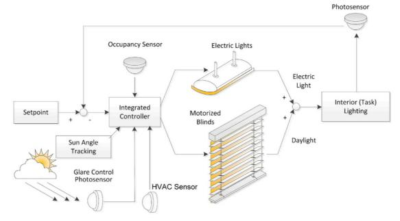
Figure 7. Fully integrated lighting and daylight control scenario. (Shen et al., 2014)
