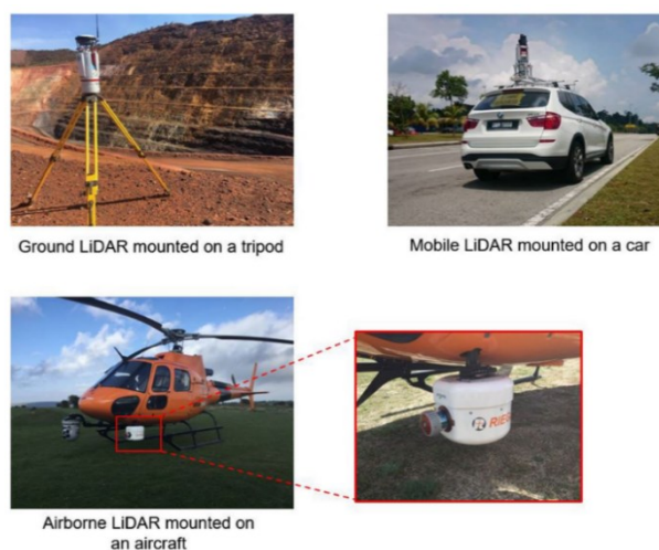
Figure 8: Examples of three types of laser scanners according to working platforms (Q. Wang et al., 2020)
