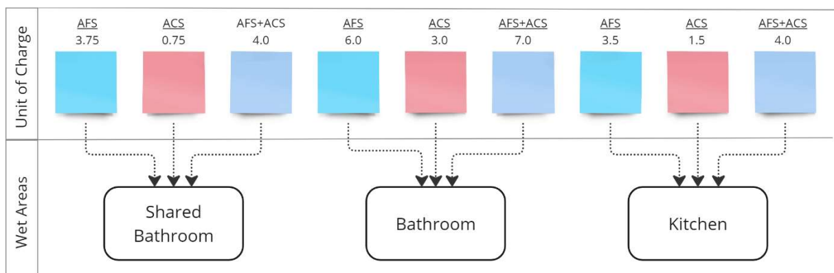
Figure 21: Water Supply Unit of Charge for Wet Areas 1 (Hot, Cold and Combined)
