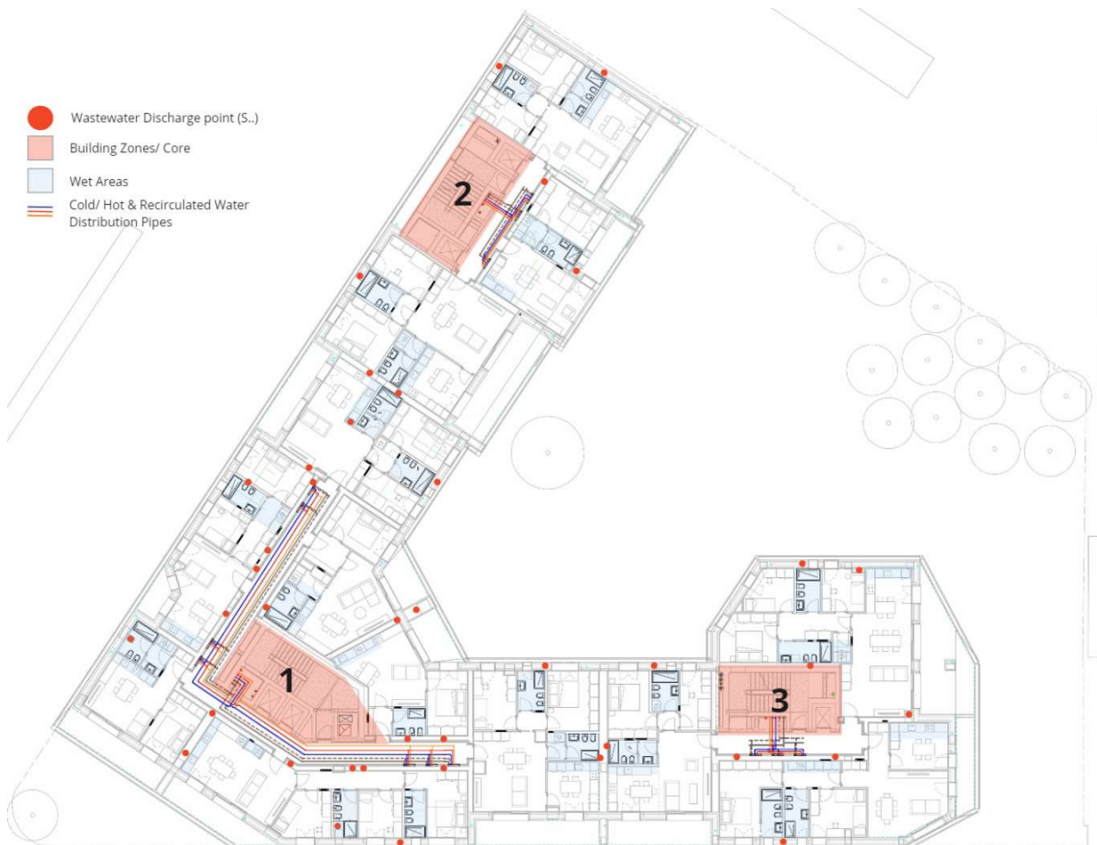
Figure 25: Level L01 showing Zones, Wet Areas, Water Supply Distribution and Wastewater Discharge Points.
