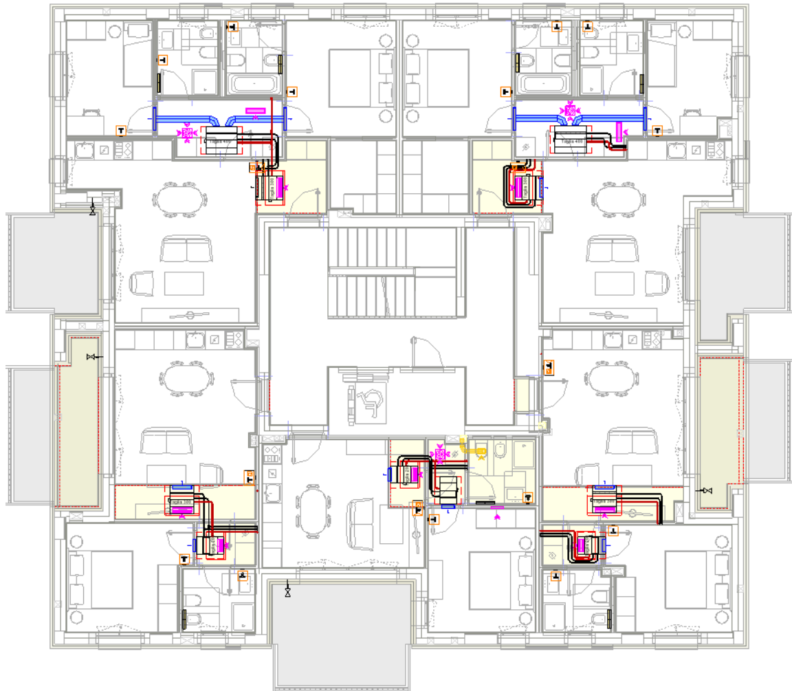
Figure 34 View of Ceiling plan shows the Fan coil location in the rooms.
