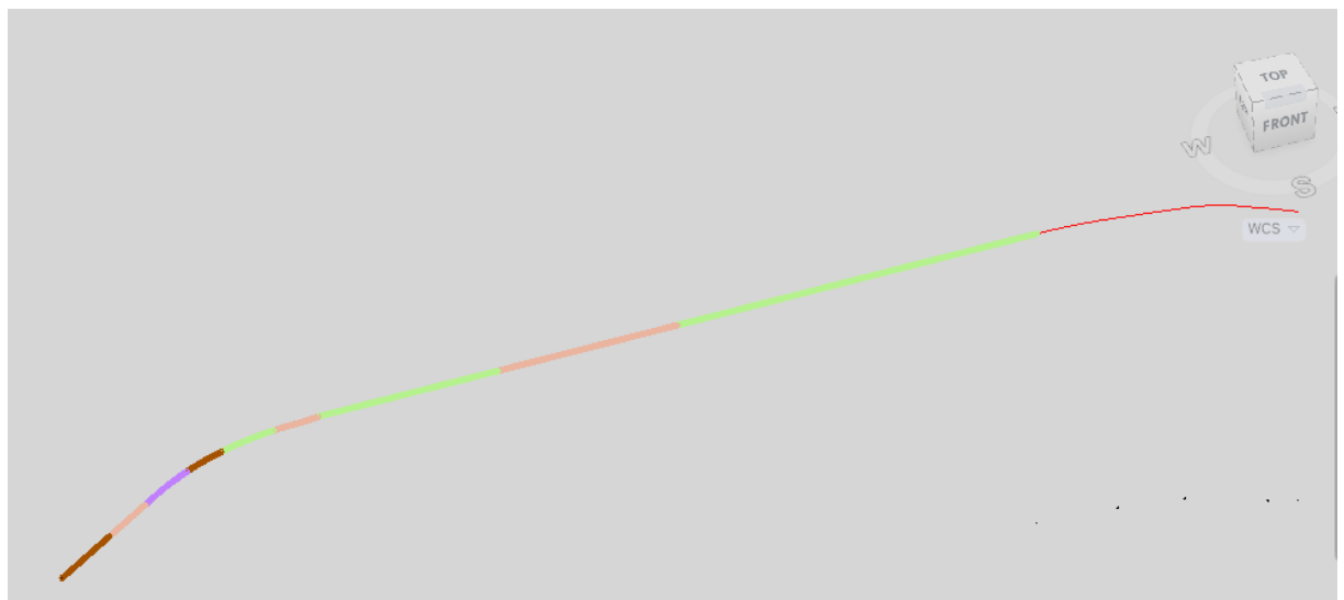
Figure 31 – Segmented alignment in Civil 3D, 3D view
