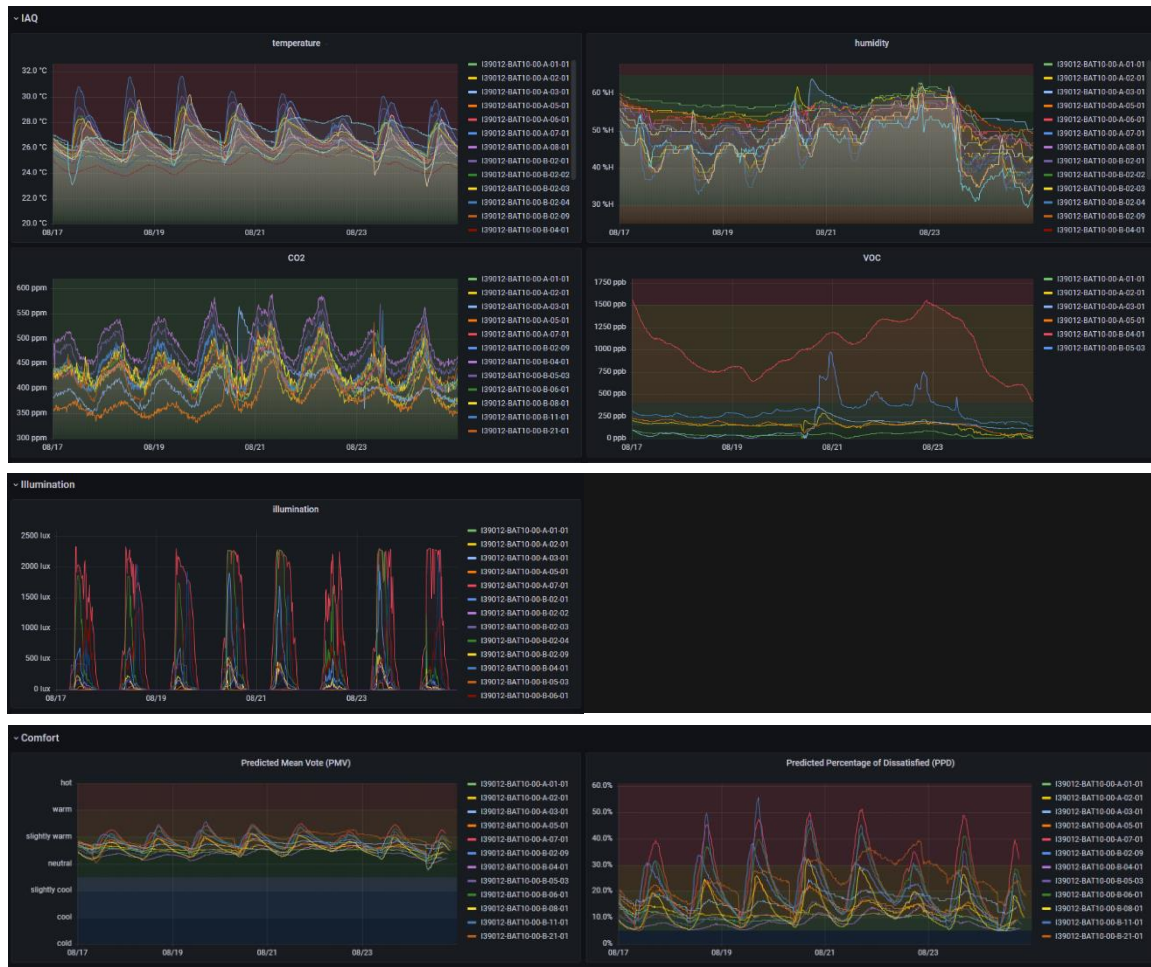
Figure 33 – Sensor data dashboard graphical represented in Grafana
