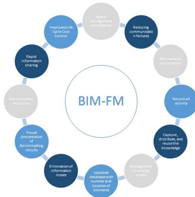
Figure 6 – Advantages of BIM-FM implementation.
