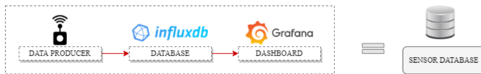
Figure 32 – Indoor Environment Data Acquisition schema
