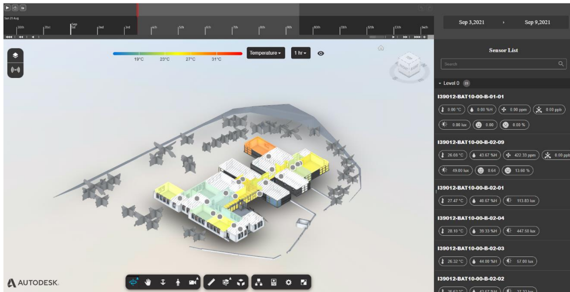
Figure 49 – 3D model displayed with heatmap surface shading data in Forge viewer
