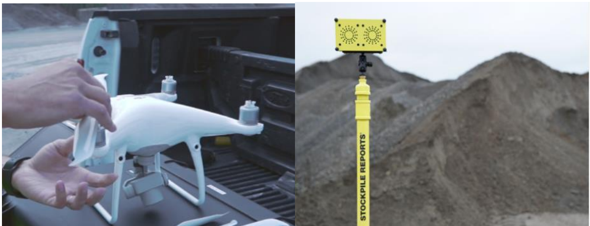
Figure 17- Using images for volume measurement (Adopted from Stockpile Reports)
